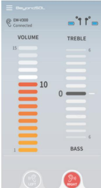
1. Use the volume control bar to adjust the overall gain. Adjust volume & treble / bass comfortably after the mode has changed. It can be saved for 4 individual modes.
